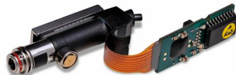
Manufactured by MPS, these pick&place grippers are based on MPS specific linear bearing technology. In order to meet the sliding force, precision, straightness and surface finish requirements set by the customer, the components are ground, then polished and finally paired with an accuracy range of 0.4  $\mu\text{m}$  using balls classed by groups of 0.25  $\mu\text{m}$ .
