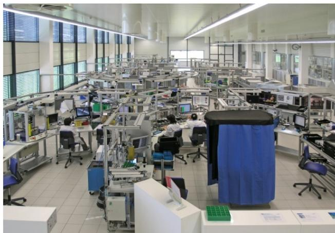
The workshop is organised according to "lean manufacturing" principles. Dedicated cells are set up when necessary.
